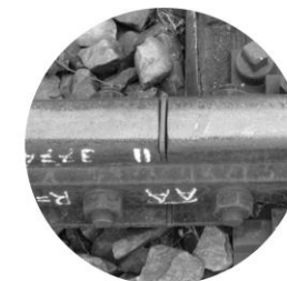
Insulated rail joints
